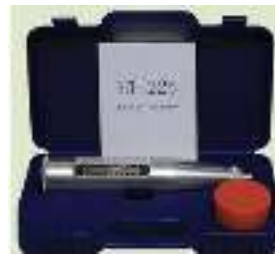
Gambar 3. Hammer Test Concrete
