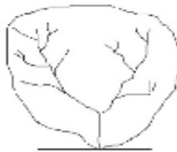
Gambar 3 Tipe DAS Paralel Sumber : (Sri Harto, 1993)
