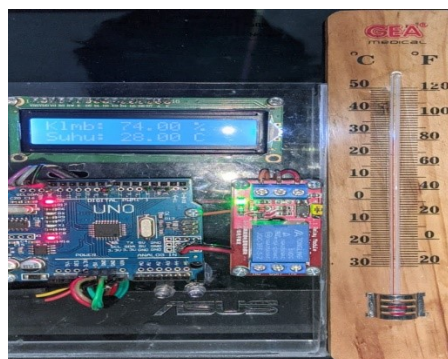
Figure 18 Calibration of Room Temperature Thermometer with DHT11
