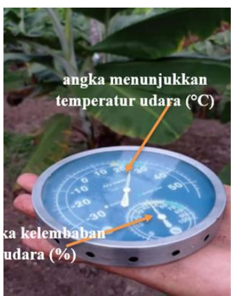
Figure 4. Anymetre TH 603 for measuring air temperature and air humidity
