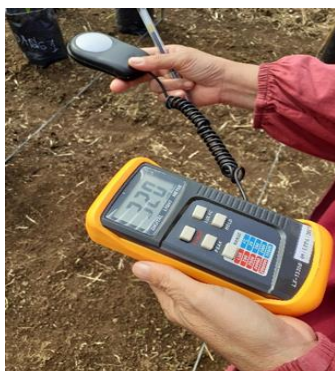
Figure 3. Lux meter LX 1330B measuring light intensity
