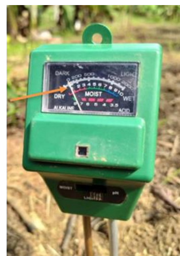
Figure 6. Soil Moisture Sensor to measure soil moisture
