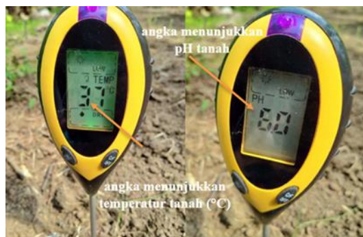
Figure 5. Soil survey instrument for measuring soil temperature and pH
