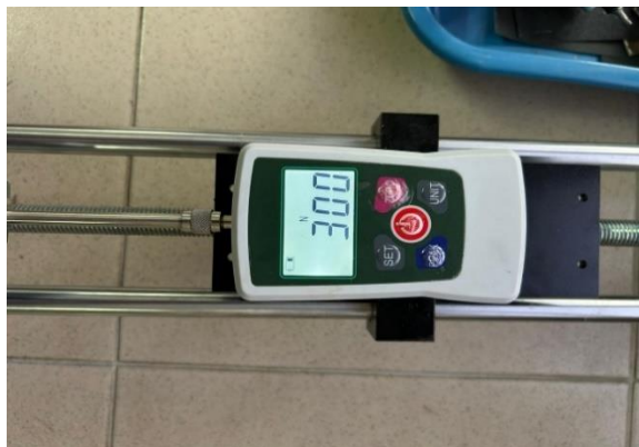
Figure 3. Settings push-pull tester for strength pull root
