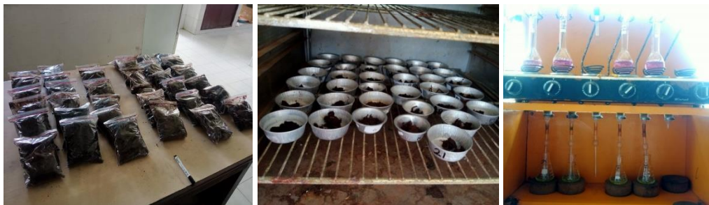
Figure 3. Documentation analysis of a sample of land peat in the laboratory
