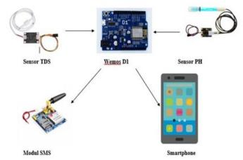
Figure 2. Internet of Things (IoT)-based Water Quality Monitoring Tool Components
