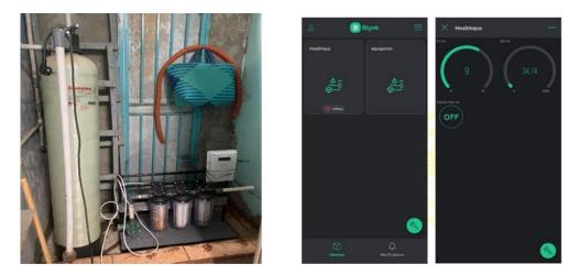
Figure 4. Addition of filters and water monitoring systems to Water Quality Monitoring devices
