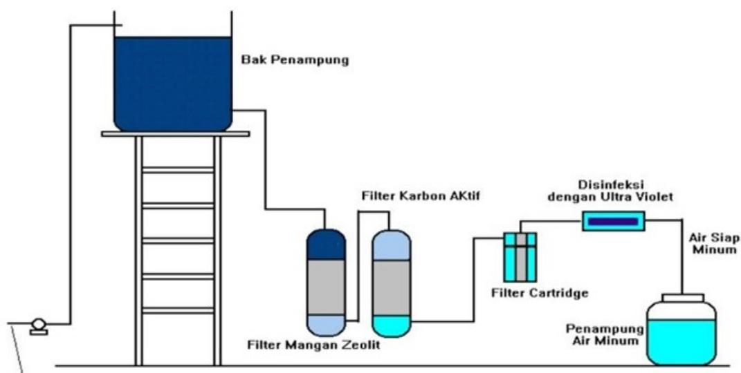
Figure 3. Physical Description of water quality monitoring equipment in the water treatment system of drilled wells into potable water based on IoT
