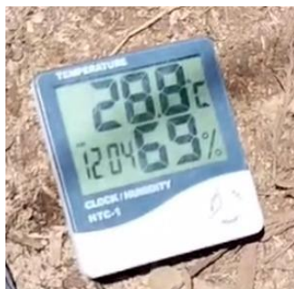
Figure 3. Measurement of air temperature and humidity
