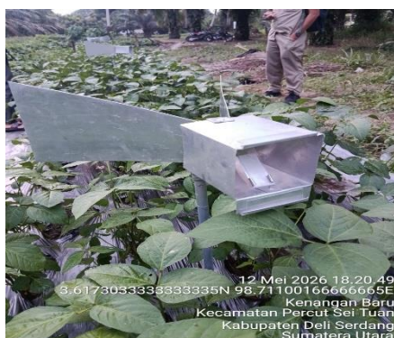
Figure 3. Photo of the spore trap tool from the research. Source: Personal Documentation (2026)
